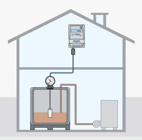
Installation of the mechanical level gauge type FSA-E via an existing, free tank connection opening
